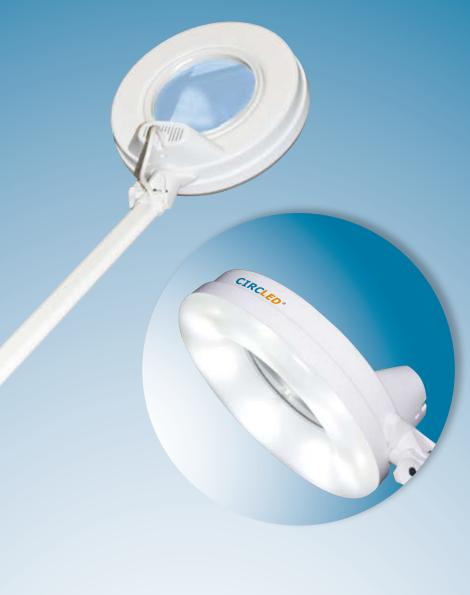
**CIRCLED** is a light suitable for countless fields of application. It is supplied with biconvex magnifier made of optical glass with a diameter of 120 mm and a magnification of 3 diopters (5 on demand).
